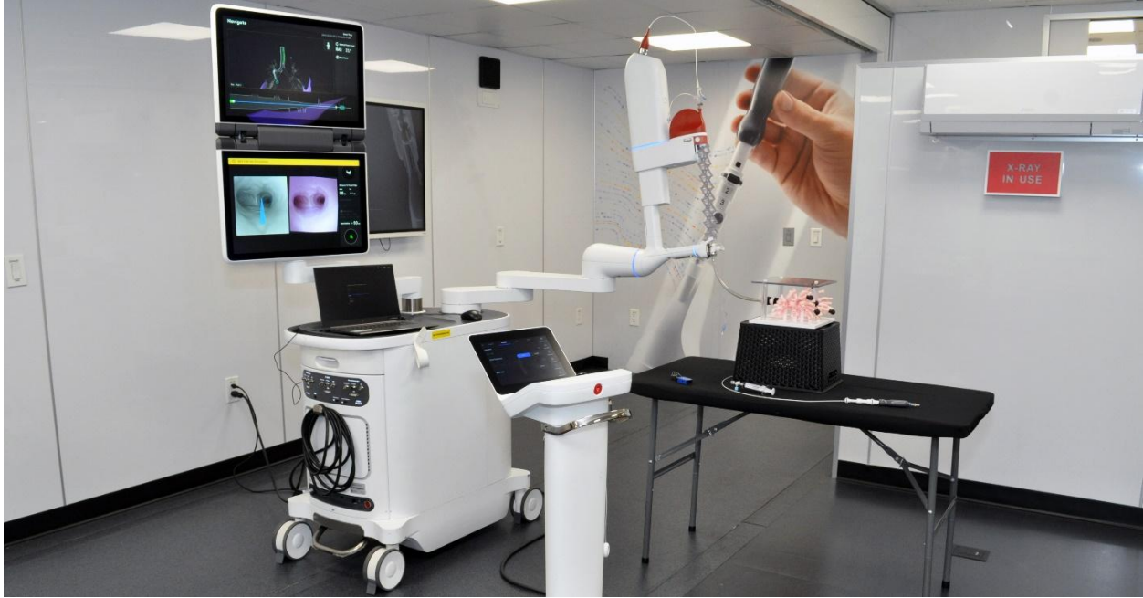
The Ion bronchoscopy robot and display screens, left; control pad, center, and bronchial system model, right
