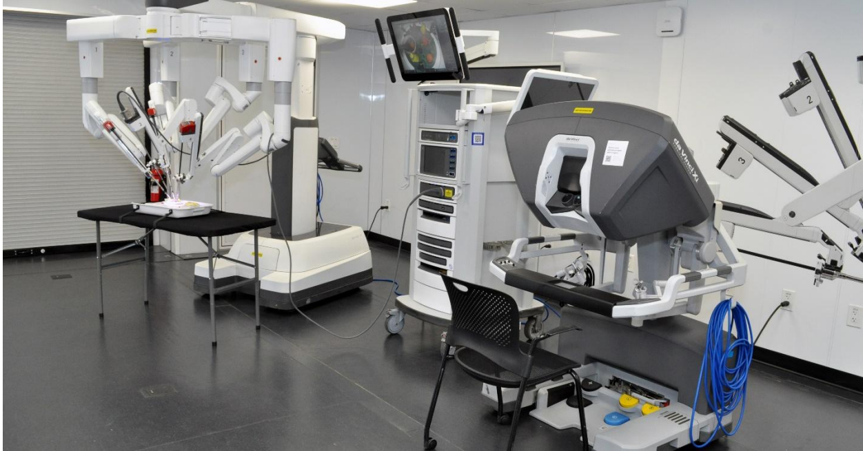
The da Vinci Si patient cart, left; computer tower and monitor, center, and surgeon's console, right
