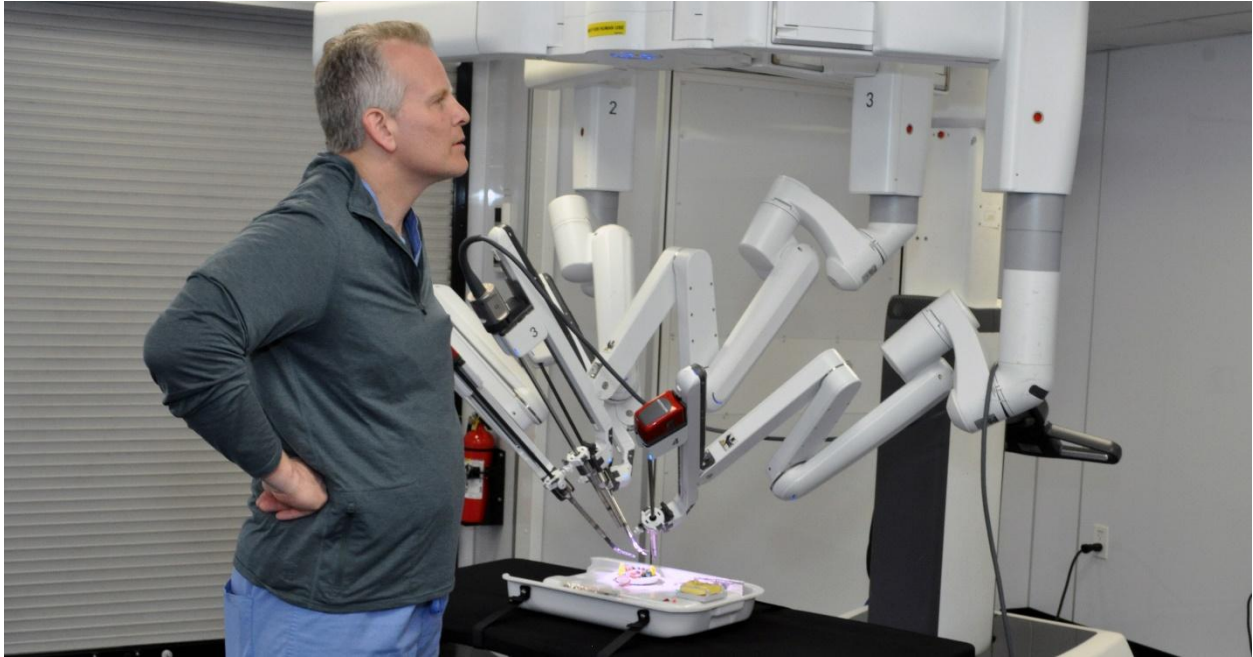
Experienced da Vinci surgeon Dr. Aaron Carr watches from the patient cart as Lab Manager Todd Tyner operates the robot
